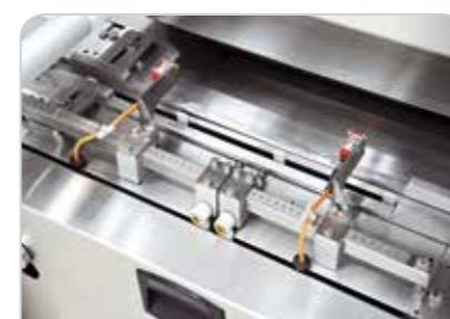
Misplaced product rejector in the infeed conveyor
